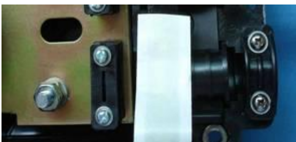
(5) Seal the unused ports by plugs.
